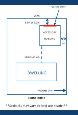
You cannot determine your property line by measuring from a sidewalk, lane or based on an existing fence. You must determine your property line through a survey or by locating your survey pins. Once you determine where your property line is, measure the setbacks from the property line.
