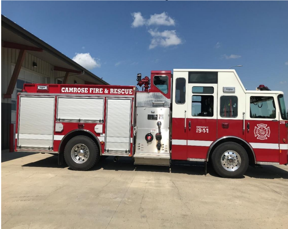
2010 Rosenbauer Custom 6000 Litre/Min Pumper (# 200)
