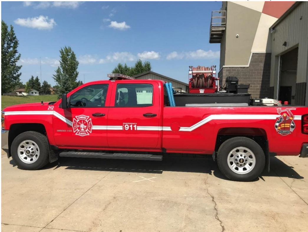
2018 Chev one-ton 4x4 Bush Truck-1350 Litre water/foam tank (# 212)
